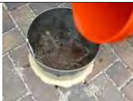
Infiltration test using ASTM C-1701
