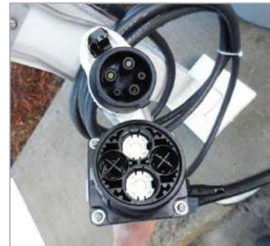
CHAdeMO connector (below) and J1772 connector (above)
